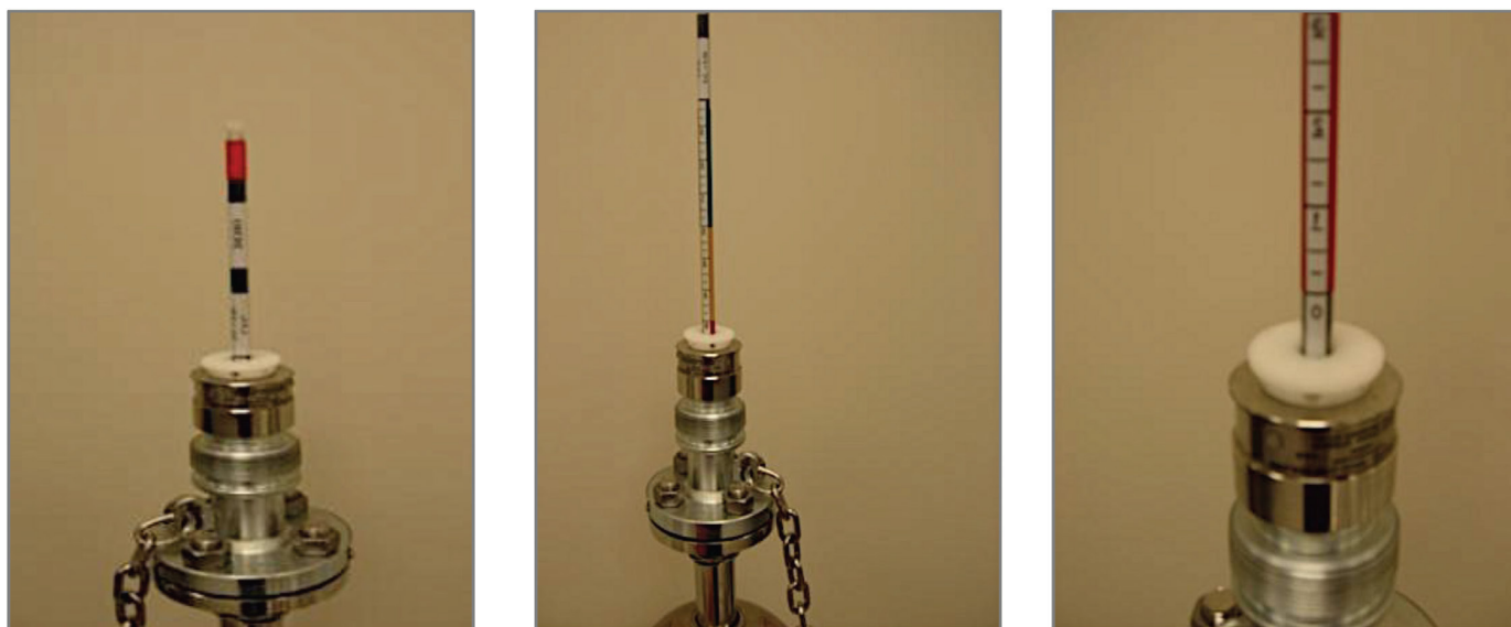
Figure 2-1 Gauge Rod Moves Upwards to Provide Level Measurement Reading.
