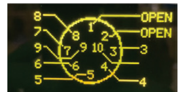
The cable connections are verified and status displayed (8870N only)
